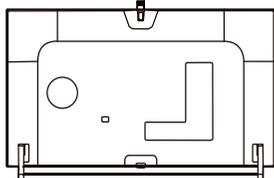
3 Push down the built-in camera when you are not using it.
